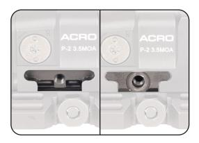
e. Insert the screw into the screw recess uf the Clamping Jaw and tighten it clockwise to approx. 1 Nm using the Aimpoint® Tool or a Torx wrench size 10.
