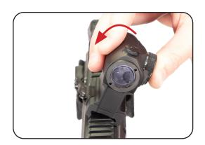
c. Close the lever to hold the assembly in place.
