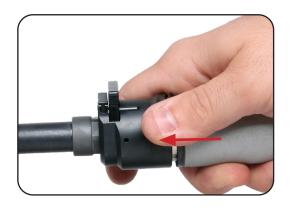
e. Push the slider down till it snaps audibly into position.
