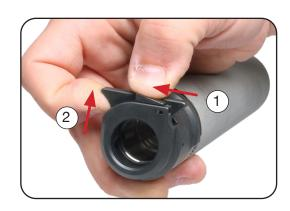
c. Loosen the suppressor body by approximately one turn in an counter-clockwise direction. If the suppressor body has already been loosened, this step can be skipped.
