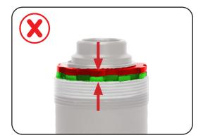
b. The cams must fit into the grooves.
