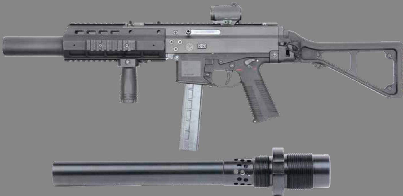
The holes in the barrel, directly in front of the chamber of the APC9-SD, reduce the pressure of the propelling gases. So normal supersonic ammunition is slowed down to subsonic speed. No expensive subsonic ammunition needed.
